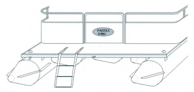
You will need: a drill with a 1/4" drill bit, a 7/16 wrench, #3 Phillips screw driver, and all enclosed hardware (4 bolts, 4 nuts, 4 over-sized washers).
